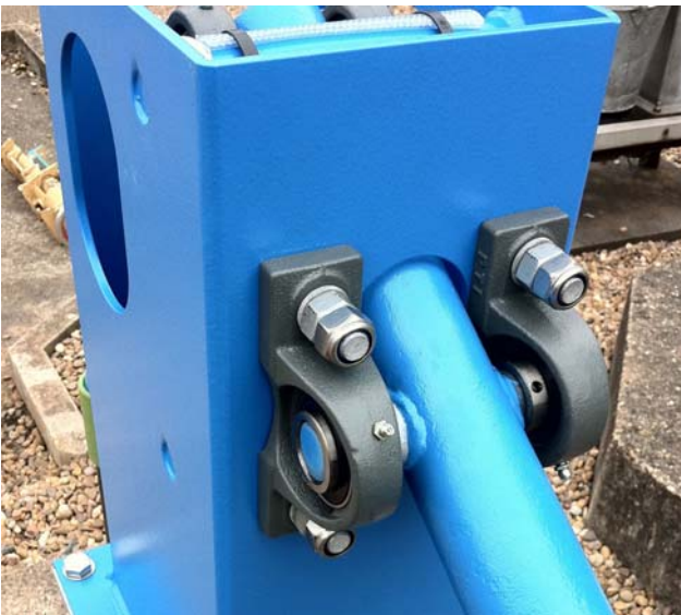
Connect the handle bearings inside out
