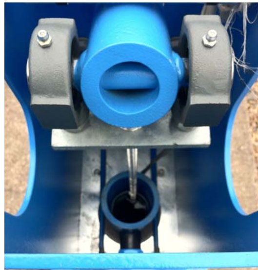
Be sure the rods move free all the way up
