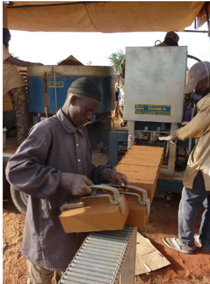
The compressed earth blocks and the machine
