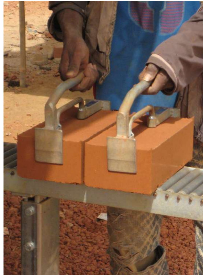
The compressed earth blocks
