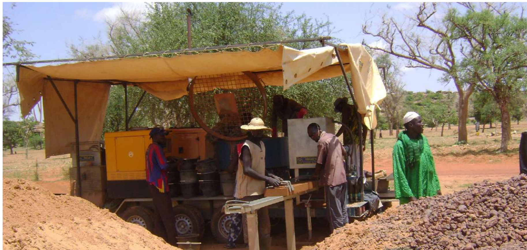
The mobile machine for the production of compressed earth blocks on site
